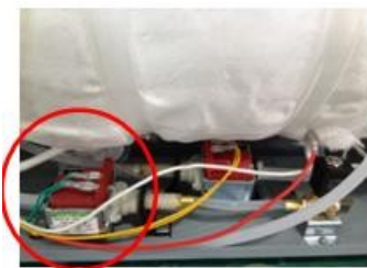
Water Pump(Green line) in the left side of sterilizer
