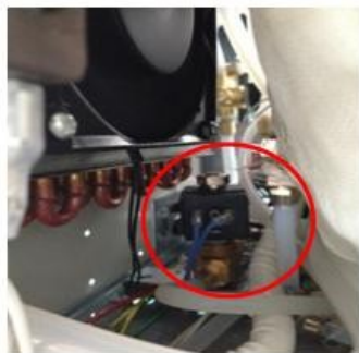
Normal-open Valve (Blue line)
