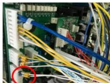
Wire line of inner sensor 2#
