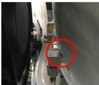
Inner sensor in the chamber bottom
