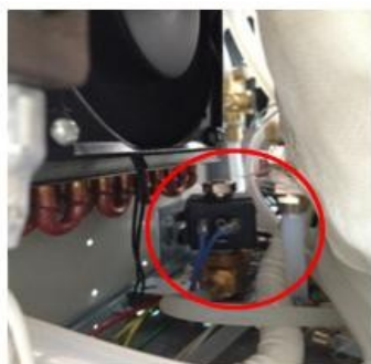
Normal-open Valve (Blue line)
